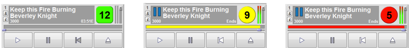
Figure 7: Cart cued with Intro of 12 seconds, Cart with 9 seconds before extro and Cart with 5 seconds before extro
